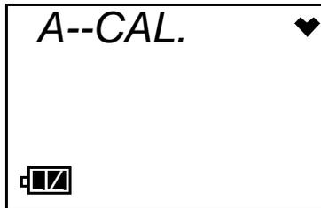
Perform a span adjustment (zero adjustment for OX-03) as part of a calibration after performing a fresh air adjustment. Performing a span adjustment (zero adjustment for OX-03)
