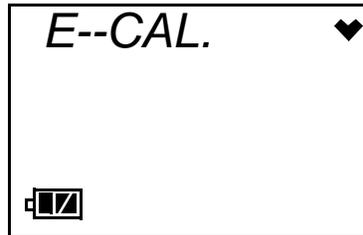
Perform a span adjustment (zero adjustment for OX-03) as part of a calibration after performing a fresh air adjustment. Performing a span adjustment (zero adjustment for OX-03) requires the use of a calibration kit. A calibration kit is available from RKI Instruments, Inc. for each 03 Series model (see “Parts List” on page 71). You will need:
