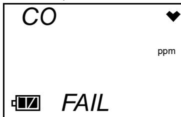
Press and release the POWER MODE button to clear the failure indication and return to the E--CAL. screen.
