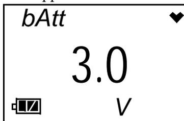
The screen displays the current battery voltage.
