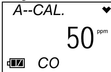
If the displayed concentration matches the calibration cylinder concentration, continue with Step 4.
