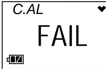
The instrument cannot be used until a successful bump test or calibration is performed. See “Calibration Mode” on page 33 for instructions.
