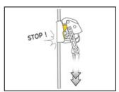
In case of a sudden movement (fall, slide, uncontrolled descent...), the fall arrester locks on the rope and stops the
