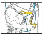
The connection arm makes the system loss-resistant when passing intermediate anchors.
