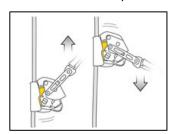
In normal use, the ASAP LOCK mobile fall arrester moves freely along the rope to accompany the user in all his movements.
