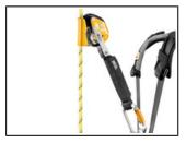
The integrated locking function allows the user to immobilize the device in order to reduce the length of a fall.
