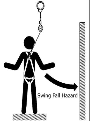
**C. FALL CLEARANCE:** Figure 2 illustrates Fall Clearance requirements. Ensure adequate clearance exists in the fall path to prevent striking an object during a fall. If the worker will be working at a position that is not directly below the anchorage point, the clearance required and vertical fall distance will be greater. The clearance required is dependent on the following factors:
