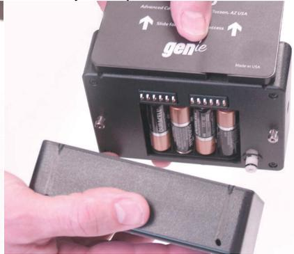
To reinstall the source module onto the base module, take the following steps: Align the air inlet fitting and the locking pins into the eyelet holes as shown. Press the two units together and slide the source module upwards (relative to the base module) to lock it in place. The two units should be flush and tightly secured at this point, then simply slide the base plate back into position until it latches.
