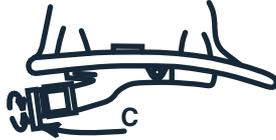
**i** When inserting suspension, front of hat can be determined by markings on the underside of the bill. Example of markings below.
