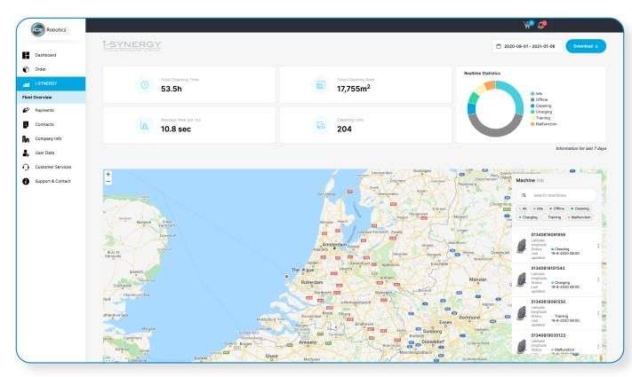
"This great smart sweeper is monitored remotely by ICE Robotics, and we don't mind that, if something goes wrong, for example a piece of plastic in the main brush which causes the brush motor to be overloaded, the system sends a notification to the technical support of ICE.
