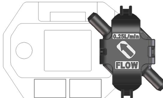
14. If necessary, use the tubing to connect the regulator to the inlet of the calibration cup.
