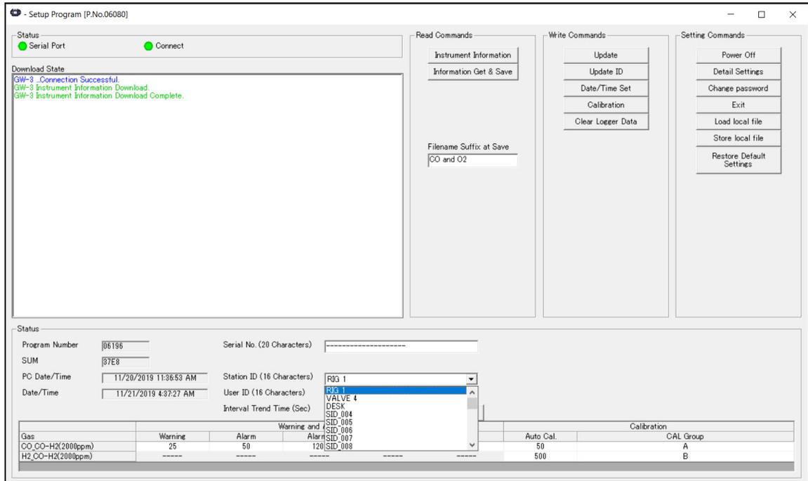
**Figure 16: Station ID Selection in Main Window**
