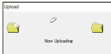
7. Click **OK** when the upload is complete. The RKI default settings are now loaded into the GasWatch 3.
