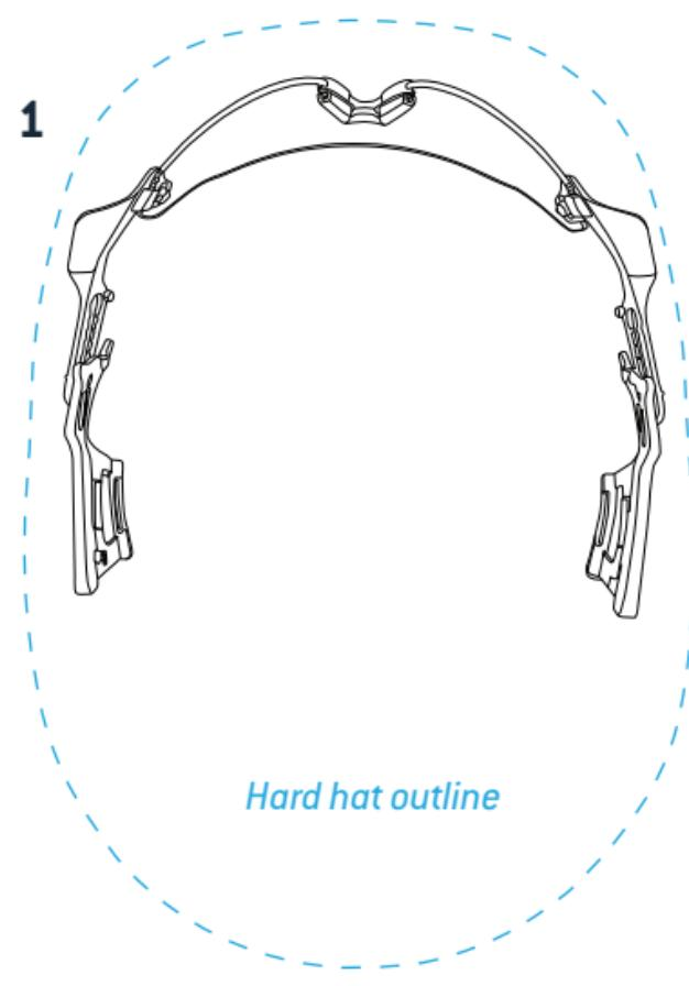
2. Clip back portion of lens accessory around suspension in the area just behind the sweat band. Repeat on both sides.
