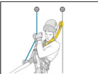
The ASAP'SORBER allows the rope to be kept at a distance, to protect it during certain work phases.
