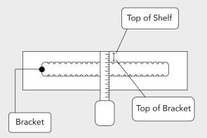
Place your bracket on the wall aligning the center of the bracket with your center line that your drew from step 3 and align the top of the bracket with the horizontal line from step 4.
