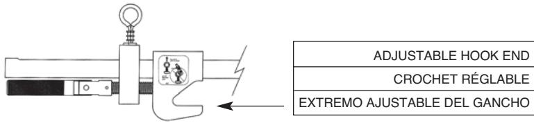
**WARNING: BE SURE ADJUSTMENT IS SNUG TO THE BEAM OR COLUMN**
