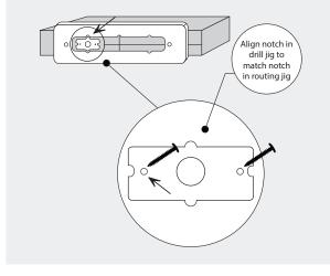
Using a power drill and an Ultra Shelf Auger Bit, drill the holes for the bracket rods.
