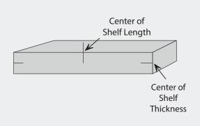
Line up the center of your routing jig to the center of your shelf for both length and thickness (notice center marks on routing jig for aligning).
