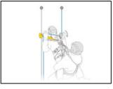
The ASAP'SORBER AXESS can be used for loads up to 250 kg in two-person rescue situations.
