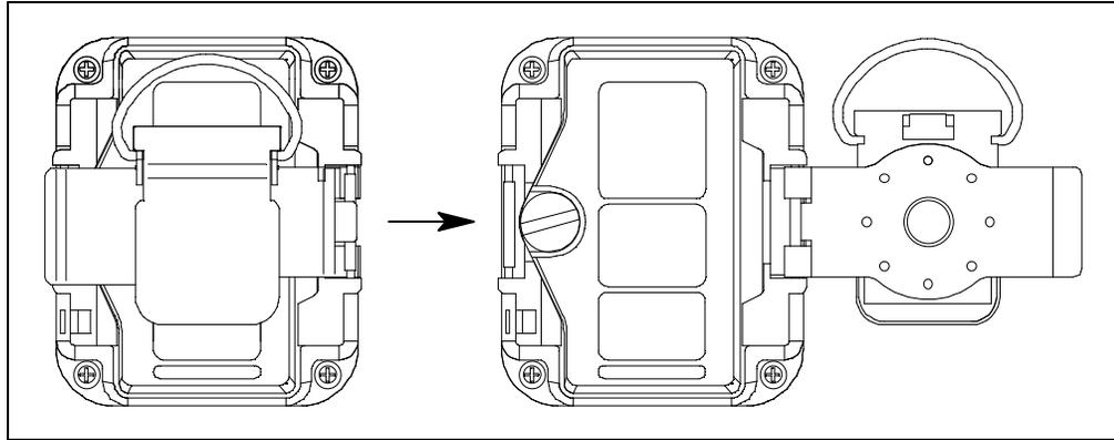
**Figure 7: Releasing the Alligator or Belt Clip**
