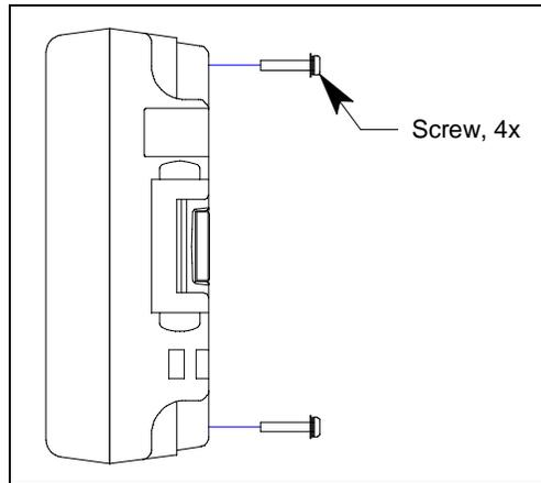
**Figure 17: Unscrewing Case Screws**
