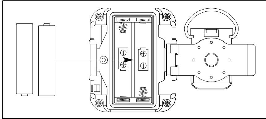
**Figure 10: Installing New Batteries**
