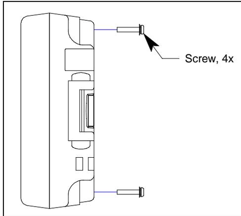
**Figure 14: Unscrewing Case Screws**
