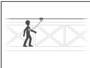
ABSORBICA-I single lanyards are designed particularly for protection on a horizontal lifeline or on an elevated platform.
