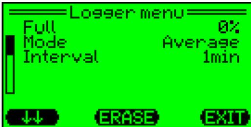
If **Interval** is selected, the data recording interval can be set between 1 second and 60 minutes by pressing **↓** and **↑**
