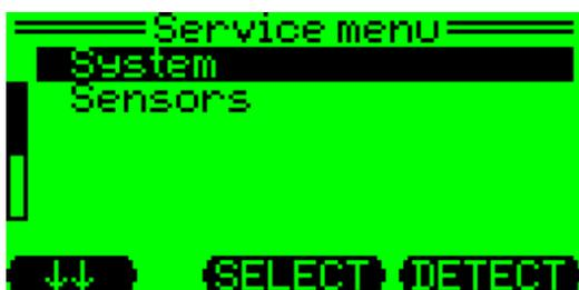
Select Sensors to adjust sensor-specific functions (alarms, calibration, etc).
