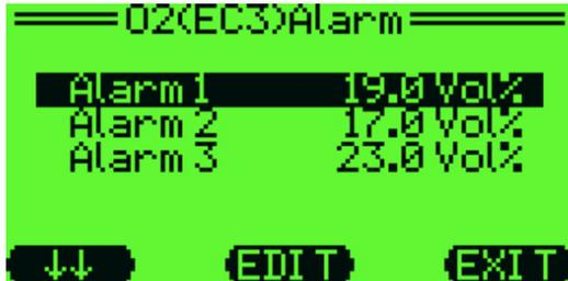
After selecting the sensor menu point Alarms the following reading is displayed (here, for an O<sub>2</sub> sensor):
